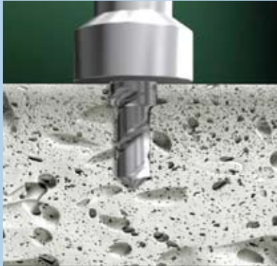
Drill pilot hole using Battery Operated Drill (BOD), hand drill, or OR drill system.
